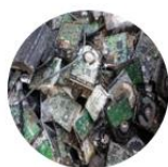
Shredded printed circuit boards (PCB)
